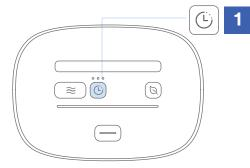
With your mask in your SoClean 3, press the **Cycle Delay** button to select the cycle delay time. The delay button will flash to indicate that the Cycle Delay can be changed.
