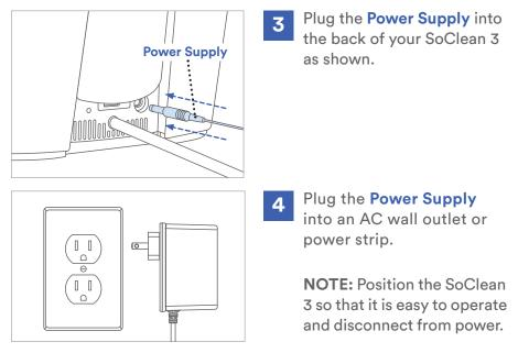
**NOTE:** Your SoClean 3 does not have a power switch to turn the device on/off. When initially connected to power, the lights on your SoClean 3 will flash a pattern that you may not see if you are not looking at the device immediately after it is connected to power. The SoClean 3 enters a low-power "sleep" mode when not in use and fully powers when you press any of the buttons on the Control Panel.
