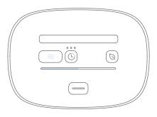
To run the Maintenance Cycle immediately, press the **Maintenance Cycle** button to start. This overrides the Cycle Delay.
