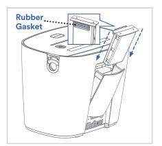
3 Insert the Filter into the slot with the blue Rubber Gasket facing the Chamber as shown.
