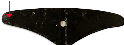
Electrode with Gel Missing
