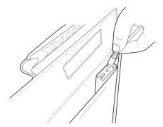
■ You can plug a Type-C USB charging cord and/or a Type-A USB cord into the Connection Box.
