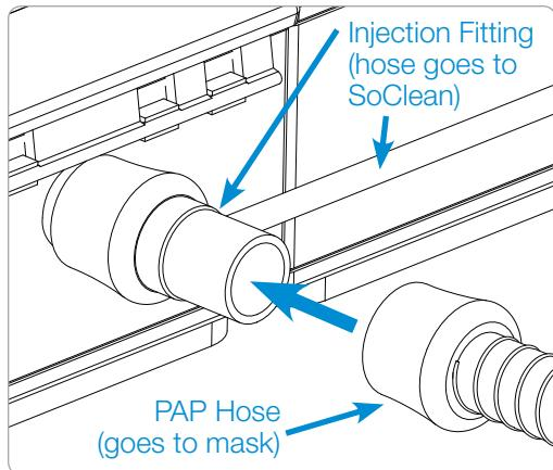
Figure 3. Connect PAP Hose to Injection Fitting
