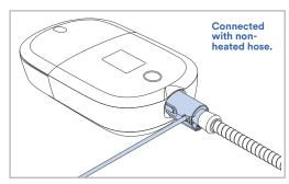
**CAUTION:** The **Ozone Tube** must be connected to the SoClean Express Adapter at all times when operating your PAP or the SoClean 2.
