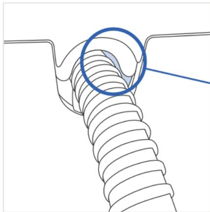
If there is visible space around the hose when placed in the Hose Slot, you may be using a 12 mm hose and require the Hose Sleeve be installed.
