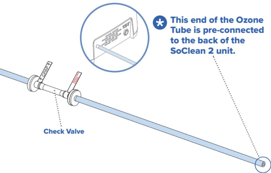
**\* This end of the Ozone Tube is pre-connected to the back of the SoClean 2 unit.**
