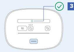
At the end of the Cycle Delay and Maintenance Cycle, the **Cycle Complete** icon  $\checkmark$  will light up **green**. You can now open the Lid and remove your mask and hose.
