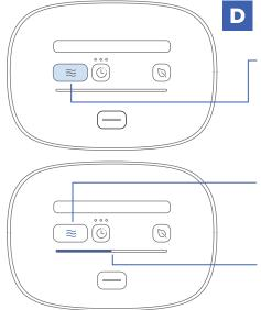
To run the Maintenance Cycle immediately, press the **Maintenance Cycle** button  $\approx$  to start.
