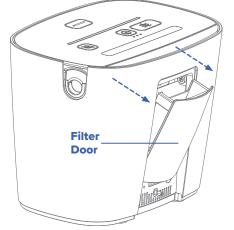
B Locate the Filter Door on the back of your SoClean unit and open it by pulling the top edge of the Filter Door away from the unit.
