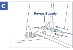
Plug the **Power Supply** into the back of your SoClean 3 as shown.
