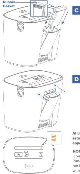
Insert the **Filter** into the slot with the blue **Rubber Gasket** facing inward as shown.
