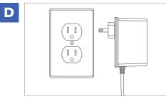
Plug the **Power Supply** into an electrical outlet or power strip.
