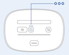
During the delay period, the **Cycle Delay** indicator lights above the button will illuminate **blue** until the Maintenance Cycle starts.
